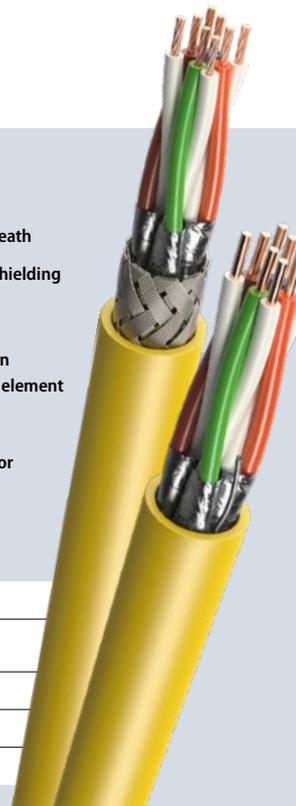
means of foil shielding or braided shielding). As a result of this cable structure, cable designs currently exist which support a frequency of 2,000 MHz. The shielded cables also meet the requirements of the new Categories 8, 8.1 and 8.2. Pair crosstalk (NEXT / FEXT) of the signals is suppressed by means of wire pair shielding. The entire shielding suppresses crosstalk between different cables installed at a short spacing from one another. This
