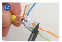
Slide the wire manager flush with the pair screen tapes and then cut the protruding wires flush with the wire manager.
