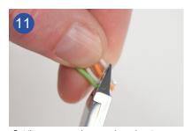
Cut the orange and green wire pairs at an angle and insert the wire pairs into the four holes in the wire manager according to the color coding (Fig. 8).
