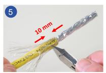
Use an electronic side cutter to cut the cable braid around the outer sheath down to 10 mm.
