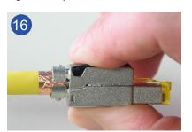
Closing the housing cover will crimp the wire manager, automatically making contact between the wires and the piercing contacts in the connector housing.
