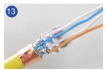
Verify the color coding and insert the blue and brown wire pairs into the guides on the wire manager according to the color designation
