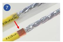
Wrap the copper foil around the braid once, snugly against the cable jacket.
