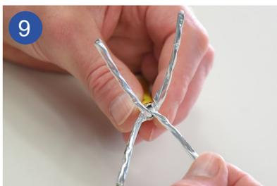
Cross out a maximum of two pairs of wires per cable end against each other in order to connect the selected coding to the wire manager (Fig. 8).
