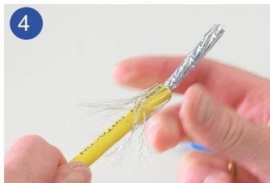
Push the cable braid back over the outer cable sheath.
