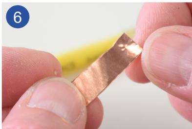
Detach the paper strip from the adhesive side of the copper tape.
