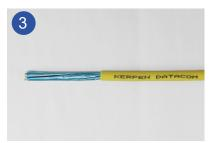
Pull off the trimmed outer cable sheath.
