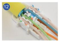
Push the blue and green wires into the grooves at the upper part of the wire manager according to the colour-code.
