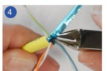
Trim the pair-insulation foils flush with the cable sheath. with an electronic side cutter.
