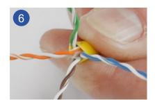
If using a cable with central cross-element instead of pair-insulation-foils, trim the cross-element flush to the cable sheath then.
