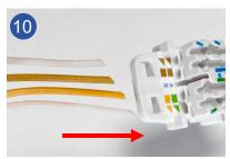
Insert the brown and orange wires into the correct slots of the wire manager according to the colour code.
