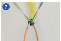
Sort the pairs according to the colour code by crossing wires (example: TIA-568B).
