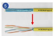
After preparing all four pairs, the cable is ready for assembly.
