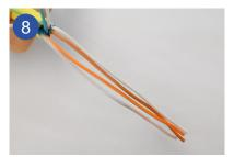
Remove the twist of the brown and orange pair and put the colours into the right order:
