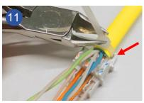
Fix the cable properly with a cable tie and cut the protruding strap.
