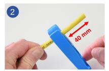
Strip approximately 40 mm of the outer jacket for the data cable using an appropriate cable stripping tool.
