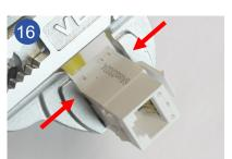
Press the wire manager firmly into the housing by using a pliers wrench until stop.
