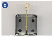
Assemble the Connect45 Pro Plus jack at the cable - make sure that there is a cable spare length of approx. 15 cm.
