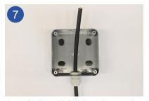
Insert the data cable into the enclosure and seal the cable gland by closing the union nut.
