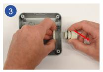
Attach one cable gland to the enclosure with the nut.
