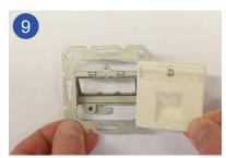
Detach the central plate from the wall-outlet and install the Connect45 Pro faceplate underneath.
